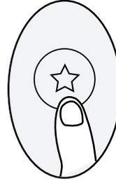
Push this button when remote controller is on, the system will automatically revert back to the previous settings including operating mode, setting temperature, fan speed level and sleep feature (if activated).
