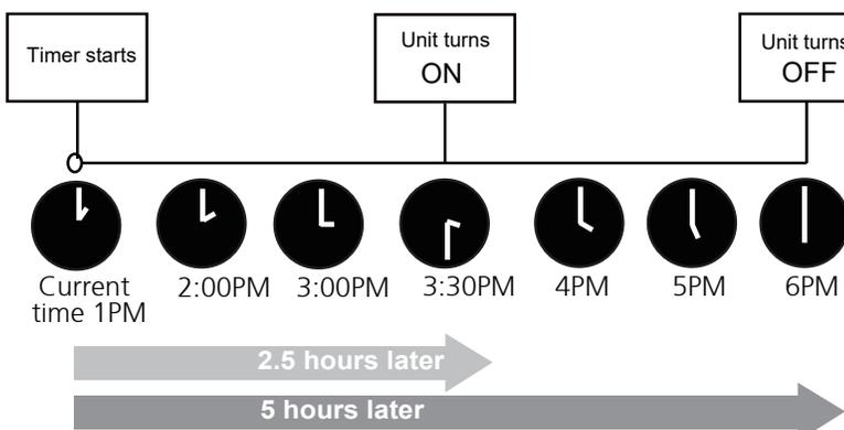
Example: If current timer is 1:00PM, to set the timer as above steps, the unit will turn on 2.5h later (3:30PM) and turn off at 6:00PM.
