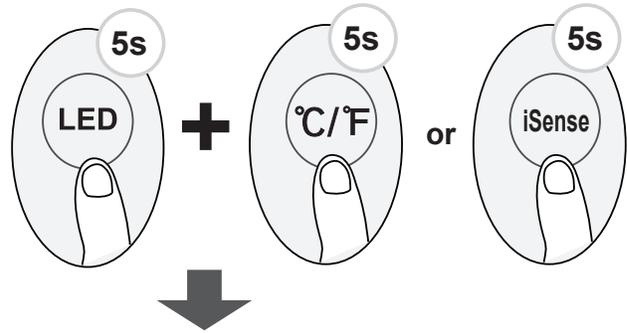
Press together **LED** button and **°C/°F** button (**iSense** button on some models) at the same time more than 5 seconds to activate Lock function. All buttons will not response except pressing these two buttons for two seconds again to disable locking.
