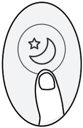
The SLEEP function is used to decrease energy while you sleep (and don't need the same temperature settings to stay comfortable). This function can only be activated via remote control.
