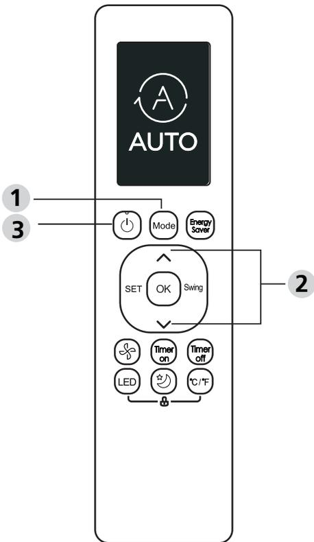
In AUTO mode, the unit will automatically select the COOL, FAN, or HEAT function based on the set temperature.
